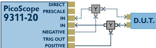
Single-ended and differential TDR setups with the PicoScope 9311-20
