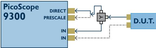
Basic setup for all PicoScope 9000 Series oscilloscopes
