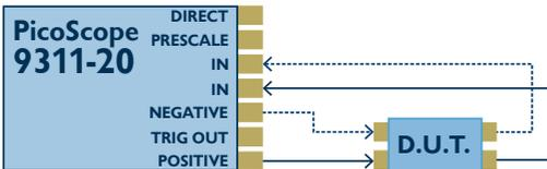
Single-ended and differential TDT setups with the PicoScope 9311-20
